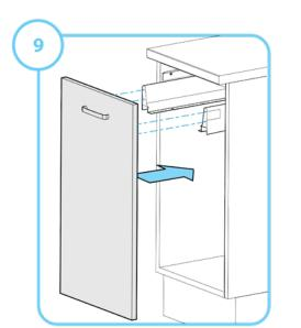
Mount door runner brackets to door and clip into the runners (screws not supplied)
